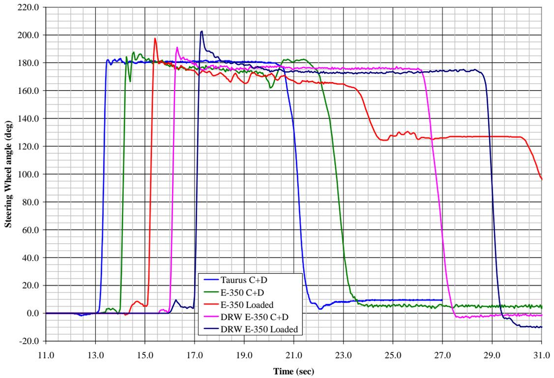
Figure 8. Slip angle response for right step steer maneuvers
