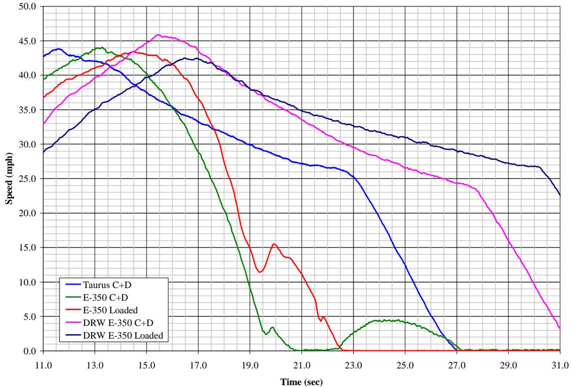
**Figure 6. Test speed input for right step steer maneuvers**
