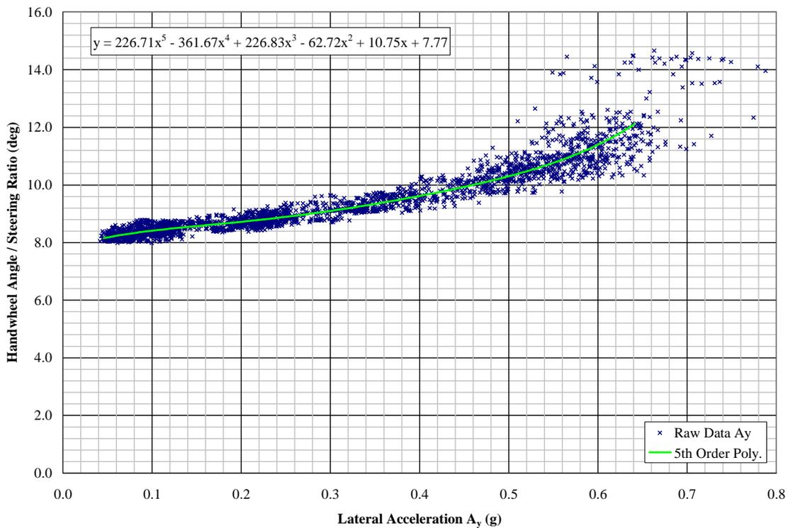
**Figure 4. Constant Radius Test Results: SRW E-350 in Curb-Plus-Driver Configuration.**
