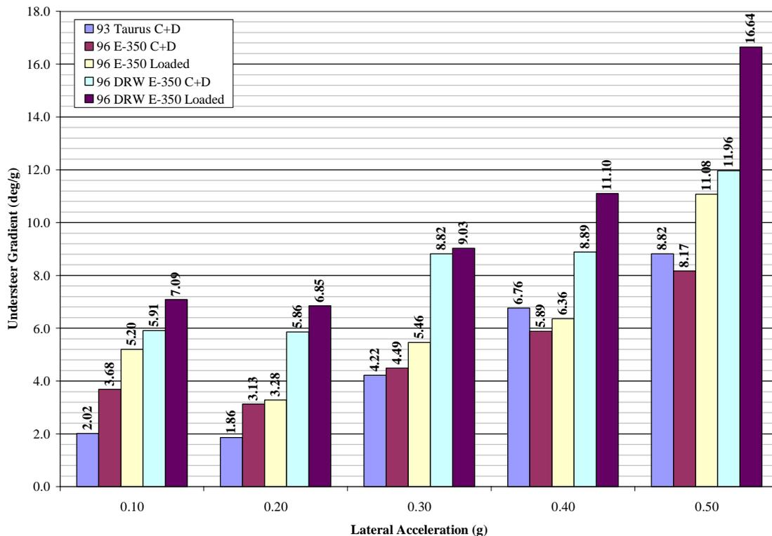
**Figure 5. Understeer Gradient Data from Constant Radius Testing**
